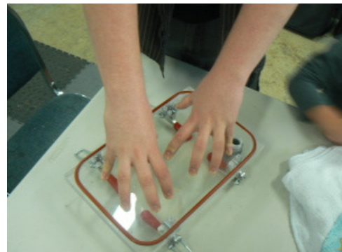
Figure 2 - Testing seal on housing lid
