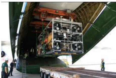
Figure 14 - Antonov 124 heavy lift transport unloading PRM
